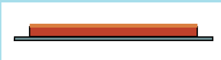
Planarize Top Surface with Flat Diamond to Establish Mirror Finish Reference Surface
